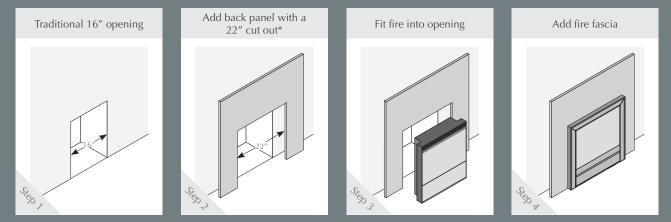
\*The Chollerton also fits a 16" back panel cut out against a standard 16" wide chimney opening with the use of a spacer frame.
