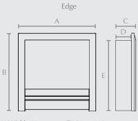
A) Width 614mm [] B) Height 611mm [] C) Depth 170mm
